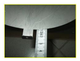
6.) Adjust the front flange plate. Very important is that the lower end of the mixing tube is around 2mm closer to the flange plate than the upper end of the mixing tube. This is the best way to guarantee that the FogMaker is tilted to the front and the condense water can flow out.
